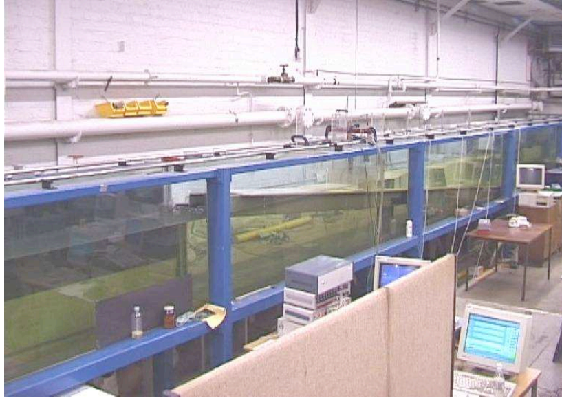
Figure 1.7: Typical example of a one-dimensional wave flume. The University of Edinburgh (photograph courtesy of Tom Bruce).
