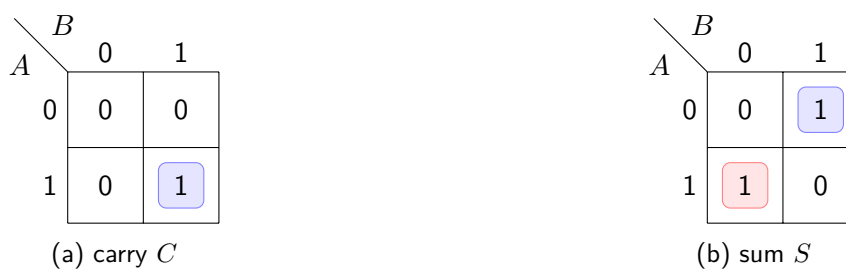
Figure 2.14: Karnaugh maps for the sum and carry column for the addition of two 1 bit numbers.
